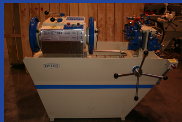
After we finish - A Refabricated Oster 784 With New Oster Die-Heads
