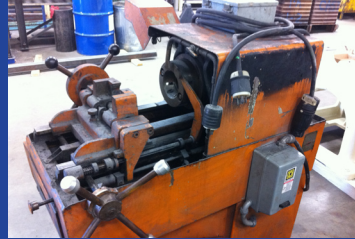
Before we get started - A used Oster 792A Rapiduction 2" Threading Machine
