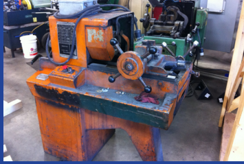
Before we get started - A used Oster 792A Rapiduction 2" Threading Machine
