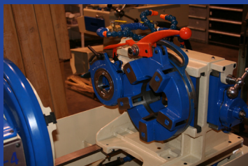
After we finish - A Refabricated Oster 784 With New Oster Die-Heads
