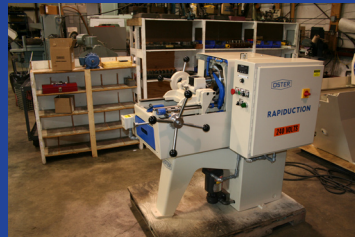
After we finish - A Refabricated Oster 792A Rapiduction 2" Threading Machine
